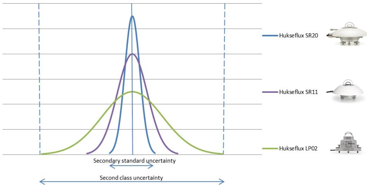
**Figure 3** A visual impression of measurement uncertainty for well maintained instruments of different ISO 9060 pyranometer classes. From second to first class and from first class to secondary standard, the achievable accuracy improves by a factor 2.
