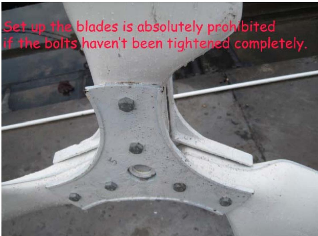
5.8 Lift the blades about 1.5m from the ground. Assemble the blades on the generator shaft, use the flat washers, spring washers, the self-locking nuts and tighten firmly.
