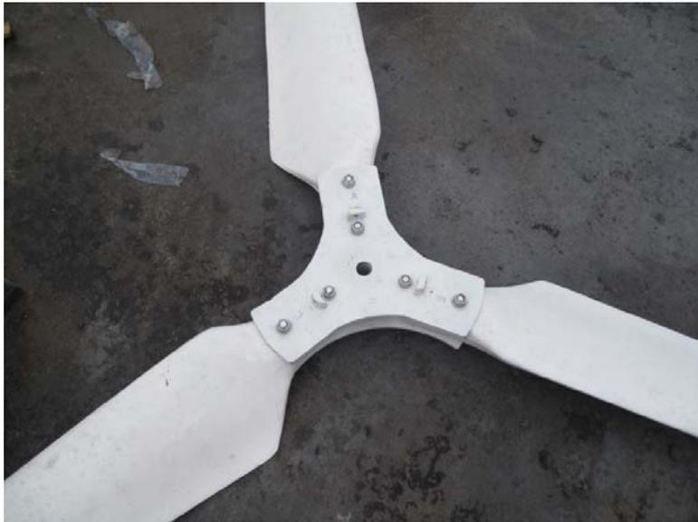
Set up the blades is absolutely prohibited if the bolts haven't been tightened completely. It will influence the balancing of one set blades.
